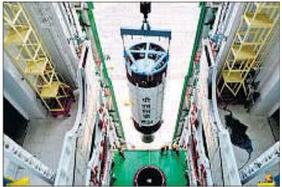
■ Hoisting of PSLV-C24 second stage during vehicle integration to carry the navigational satellite IRNSS - 1B, in Andhra Pradesh PTI PHOTO
